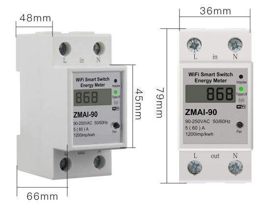
Note: This Power Meter needs Neutral line and Live line to install. Install 35mm Din Rail
